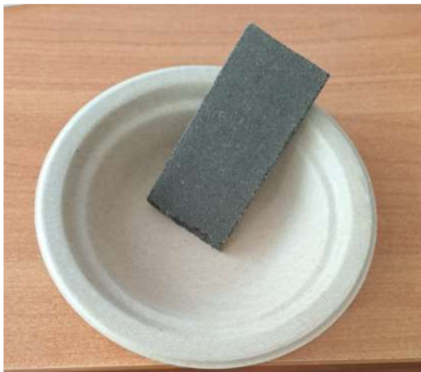
Fuel pellets and disposable tableware made of reed
